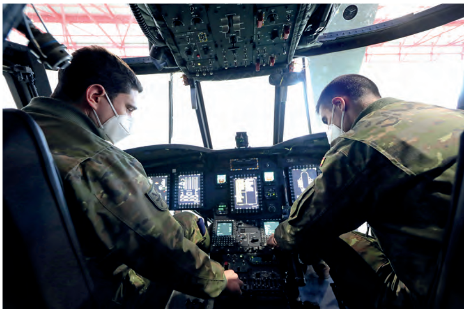
The on-board equipment is digital and the two pilots have five screens that provide them with the data and information necessary to control the flight.
