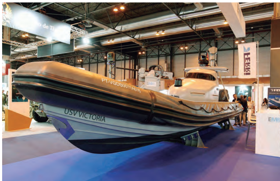
The USV Victoria remote control naval platform by Ferry configured with the Sentinel 12.7 mm remote control tower and the OTEOS camera, both by Escribano.
